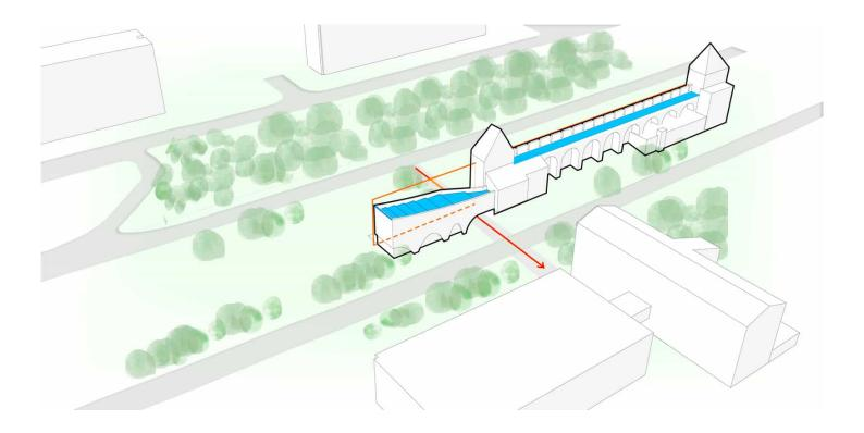
Due to the continuation of the city wall's arches, the passage Blaue-Funken-Weg could be retained. A bridge, which becomes a part of the building, provides access to the existing structure. The accessibility is comparable to the city wall walkway.
